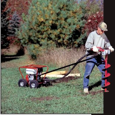
ittle Beaver earth drills are incredibly fast. Operating at 360 RPM's, our augers rotate much faster than competitive units. Not only does this increase your drilling productivity, but it also results in cleaner holes.
